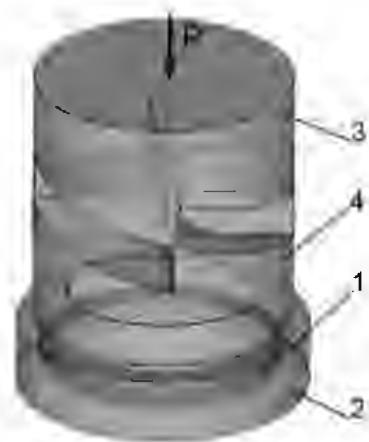
1 – workpiece, 2 – glass, 3 – punch, 4 – deforming element
